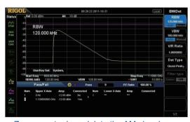
Zero span to demodulate the AM signal
