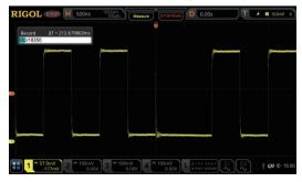
Adopt the segmented storage technology, you can set the trigger conditions to make a selective choice in capturing and saving the signals that you are interested in
