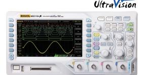
DS1000Z Series is the high performance, economic level general purpose oscilloscope which provides 4 analog channels, the bandwidth from 50MHz to 200MHz, up to 1GSa/s sample rate.In particular, DS1202Z-E is dedicated for online sale. It has two analog channels, with the bandwidth of 200 MHz. With the Ultravision technical platform, the DS1000Z series has sustained its characteristics of deep memory and high capture rate, exhibiting its cost-effective advantages.
