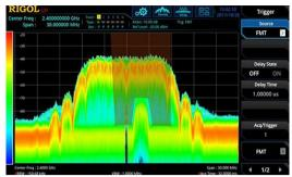
The FMT frequency mask trigger is a unique trigger mode for real-time spectrum analyzers. You can quickly build a template and accurately locate and trigger signals that match the template rules to detect sporadic anomalies within the monitored range.
