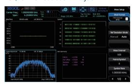
ASK/FSK demodulation analysis software can help engineers demodulate and analyze signals such as TPMS, PKE/RKE, and obtain parameters of signal modulation quality to help products get listed quickly.
