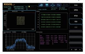
The VSA supports a variety of digital modulation formats such as QAM, PSK, MSK, ASK, FSK, etc. This function is used to quickly demodulate and display multi-dimensional data such as its constellation, eye diagram (baseband signal), spectrogram, demodulation data, etc., to discover problems in the design.
