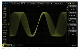
The intensity graded color display capability provides the fluorescent display effect, making the waveform changes obviously to be seen.
