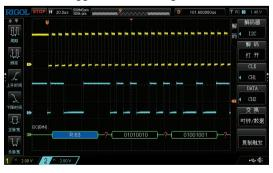
Provide bus trigger and decoding options, support RS232/ UART, I2C, SPI bus.
