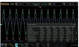
DS8000-R, MSO8000series, MSO/DS7000 series and MSO5000 series oscilloscopes support the optional built-in power analysis software, which can complete the power quality analysis and ripple analysis. The power analysis software can help engineers analyze the commonly used power parameters rapidly and accurately, without needing to make tedious configurations manually or do complicated formula calculation.
