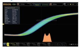
Measurement histogram is applicable for observing the distribution of the measurement signal over a long period of time to help users quickly find out the potential abnormalities of the signal.
