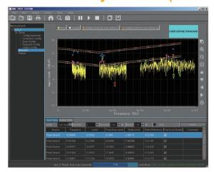
EMI Test System is a PC application software developed by RIGOL for RSA5000, RSA3000/E, DSA800, DSA800E and DSA700 series with the EMI-DSA800 option to do the EMI Pre-compliance tests.
