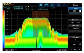
The FMT frequency mask trigger is a unique trigger mode for real-time spectrum analyzers. You can quickly build a template and accurately locate and trigger signals that match the template rules to detect sporadic anomalies within the monitored range.
