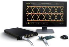
A single device with peripherals can meet traditional oscilloscope applications: connect the display device through the HDMI interface to view the user interface, connect the mouse through the USB Host interface to click and drag, and connect the keyboard to set numbers or strings.
