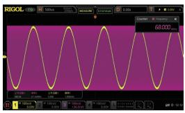
Measure accurate frequency value of the waveforms based on memory, not the screen display.
