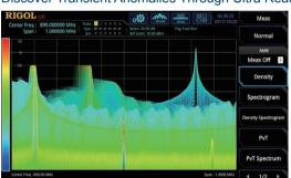
The RSA5000 series delivers up to 40MHz of real-time bandwidth using the original Ultra Real technology. In the real-time bandwidth range, transient signals exceeding 7.45us duration can be guaranteed to be 100% captured and accurately measured.
