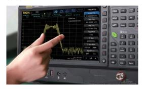
You can use the RSA5000 series to provide a 10.1-inch capacitive multi-touch screen for quick setup, and support a variety of gestures such as dragging, expanding, and zooming waveforms to provide a personalized interactive experience that maximizes your time.
