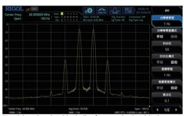
Resolving signals with similar frequencies is critical to verifying many RF devices and systems. With the RSA3000E, the RBW resolution bandwidth with a scan bandwidth of only 1 Hz allows you to view more details of adjacent signals.
